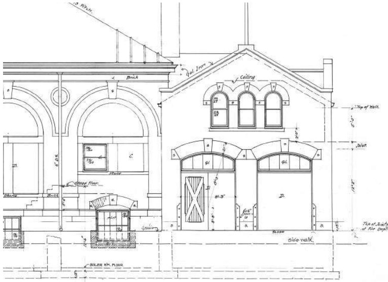
Photo10: Original drawing showing the door configuration, windows above doors, infilled with existing material.
